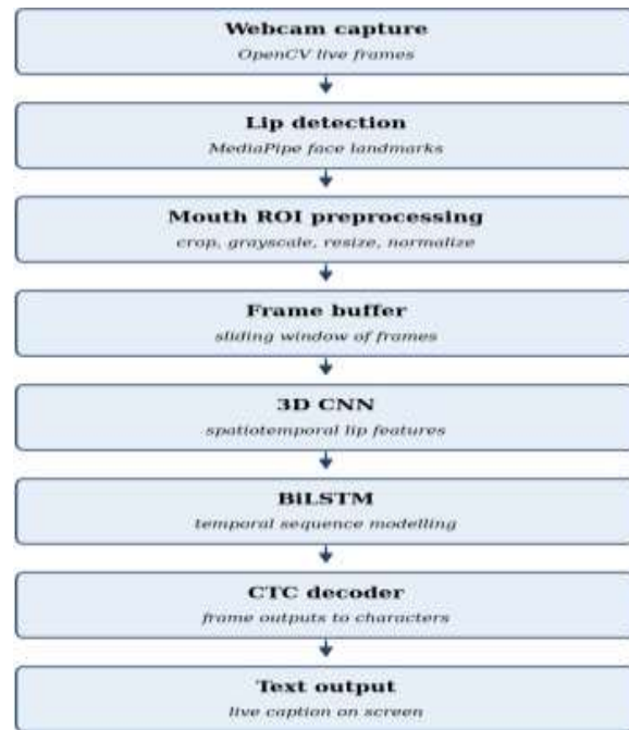
Fig. 1. Functional block diagram of the real-time lip-reading system.
