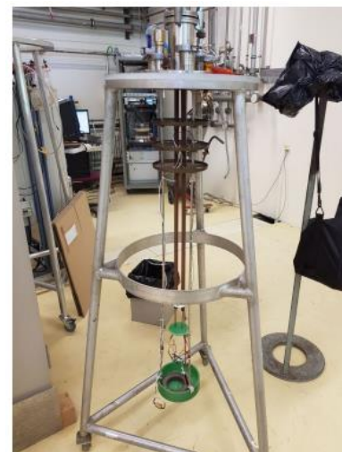
FIGURE 3.12: Sample installed in the cryostat.
