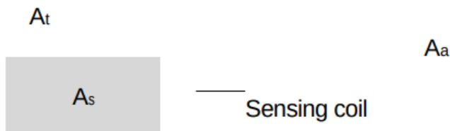
FIGURE 3.2: Representation of the cross-sectional area of the sample A_s and of the sensing coil A_a . The cross-sectional area of the air gap is A_s = A_t - A_s .
