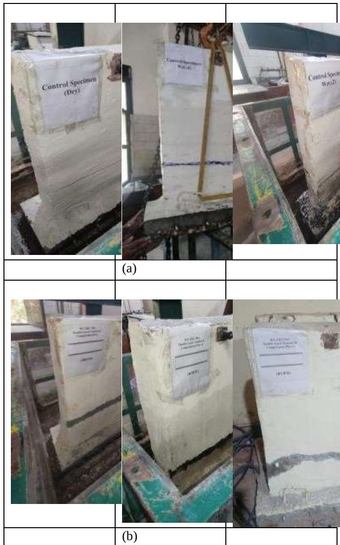
Figure 6: Comparison of the observed failure patterns of (a) unstrengthened control specimens and (b) BTRM-strengthened specimens.
