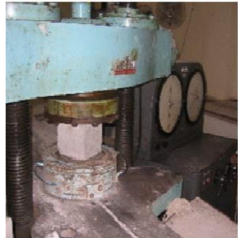
Fig. 7. Cubes tested for compressive strength.
