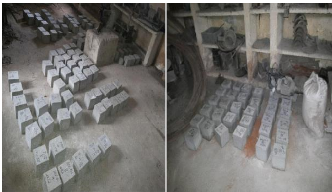
Fig. 6. Specimens kept for curing.
