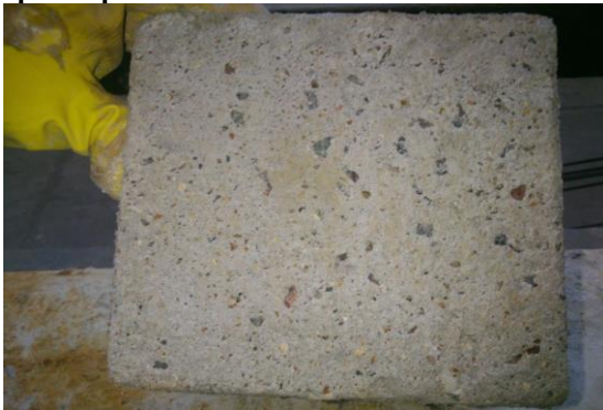
Figure 9 “Specimen of normal SCC immersed in 5% HCl”
