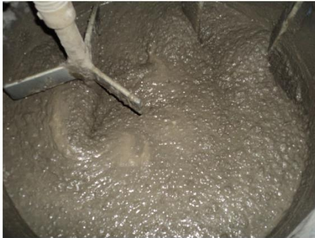
Fig. 5. Self-compacting concrete after mixing in 120 kg pan mixer.
