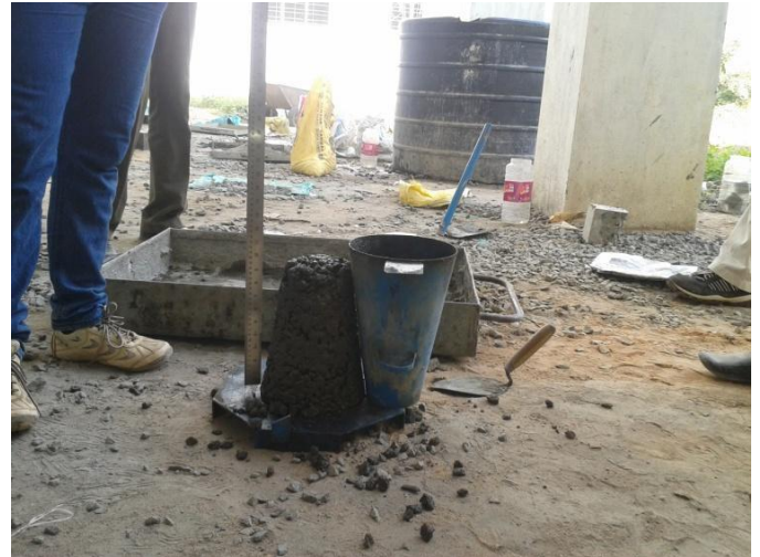
Figure 2. Slump cone test on concrete.
