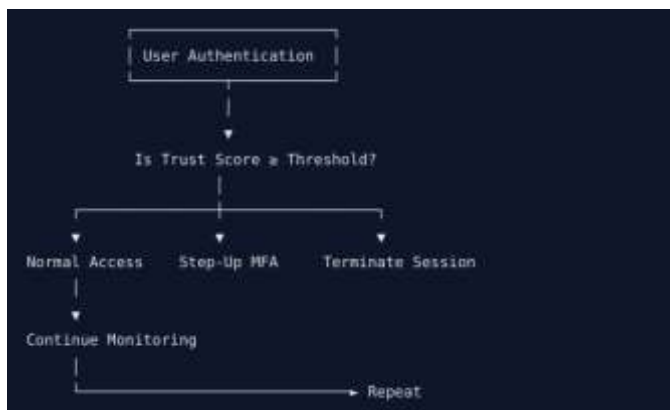
Figure 2. Continuous authentication workflow of the proposed ATCAF framework.
