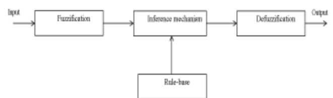
Figure 10. Schematic Diagram of the fuzzy logic controller
