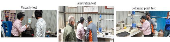
Figure 1: Actual laboratory testing of VG-30 bitumen used in the study
