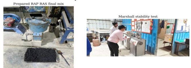
Figure 2: Actual preparation and Marshall testing of the RAP RAS asphalt mixture
