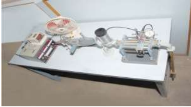
Setup of microwave X-band for measurement of dielectric properties.
