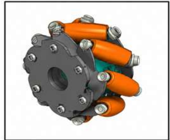
Fig 3: A Mecanum Wheel
