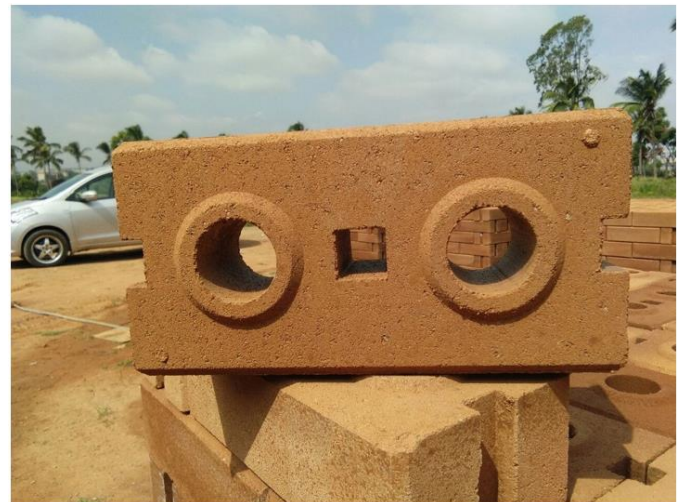
Figure 6. Stabilized compressed earth blocks (CEB) and a rammed earth wall section. Adding 5–8% Portland cement or hydraulic lime to compressed soil raises compressive strength to 3–5 MPa while retaining thermal mass and low embodied energy.
