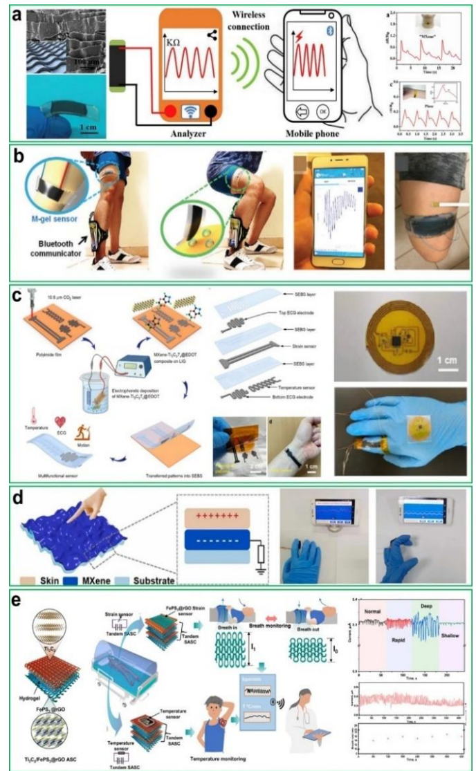
Fig. 7. (a) Polyaniline@Ti3C2-based flexible strain sensor with a tile-like stacked structure for wireless detection of artery pulse and phonation [77] (b) Wearable wristband based on a Ti3C2 hydrogel strain sensor and Bluetooth module wrapped around a human thigh during a workout to measure the degree of muscle tiredness [78] (c) Ti3C2@3,4-ethylenedioxythiophene/graphene composite-based wireless multifunctional sensors for strain, temperature, and heartbeat monitoring [79].
