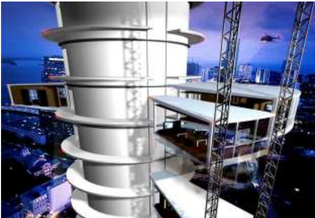
Figure 2. Conceptual illustration of a prefabricated floor module showing the steel platform, cantilevered edge, façade panels, and integrated MEP runs. In a rotating tower, multiple such modules are stacked around the central core and attached to the rotation mechanism.
