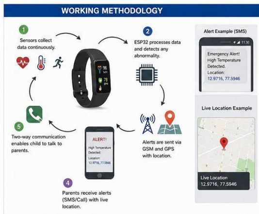
sensors. The MAX30100 pulse oximeter and heart rate sensor monitor the child’s heart rate and oxygen level, while the LM35 temperature sensor measures body temperature. These sensors continuously transmit real-time data to the processing unit for analysis. Fig 2: Working Methodology
