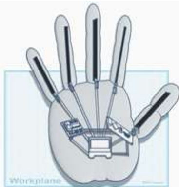
Fig. 1: Design representation of the wearable hand gesture vocalizer glove.
