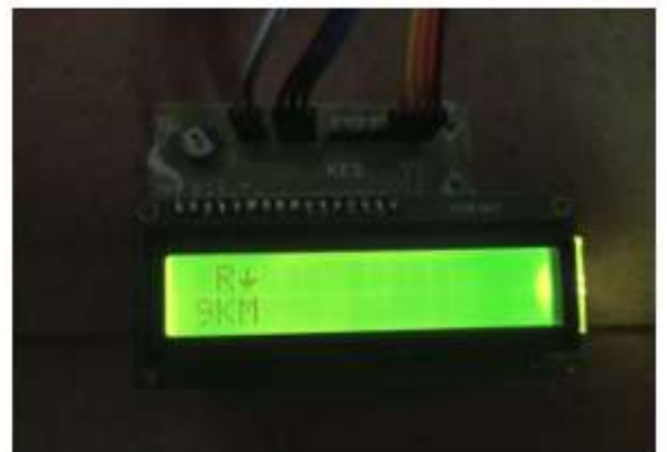
Fig. 8 Fault Indication at 9Km distance
