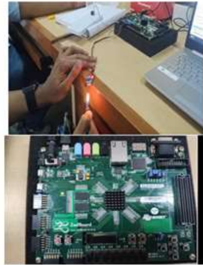
Fig. 2. Experimental setup of an FPGA-based home automation system
