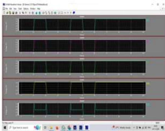
Fig. 8. Output waveform of GDI 4-bit full adder
