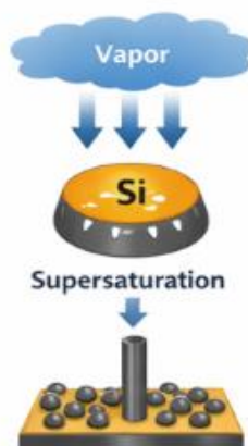
VLS Nanowire Growth Mechanism
