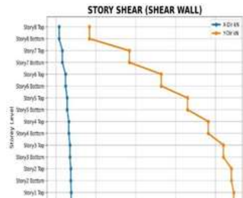
Fig. 18. Storey Shear – Shear Wall Structure
