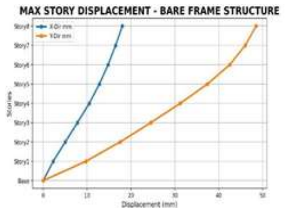
Fig. 13. Maximum Storey Displacement – Bare Frame Structure
