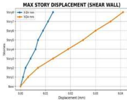
Fig. 15. Maximum Storey Displacement – Shear Wall Structure
