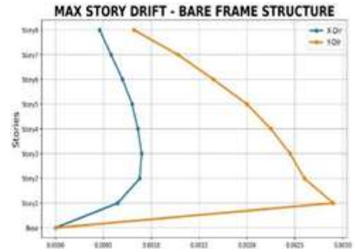
Fig. 7. Maximum Storey Drift – Bare Frame Structure
