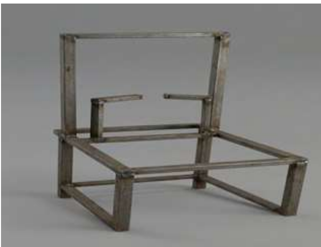
Fig 7.2: Mild Steel Metal Frame
