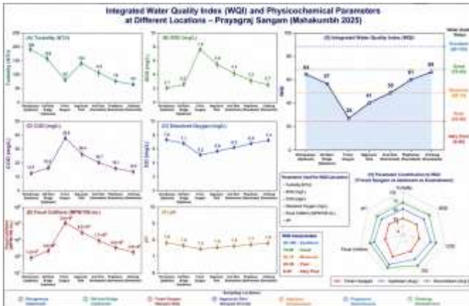
Fig. 3. (a) Integrated Water Quality Index (WQI) and Physicochemical Parameters at Different Sampling Locations in the Prayagraj Sangam Region During Maha Kumbh 2025
