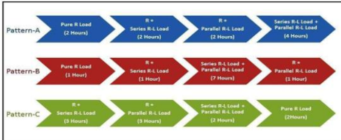
Figure 12: Three Sample Load Patterns for Monitoring
