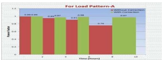
Figure 13: Power Factor Variation for Load Pattern A
