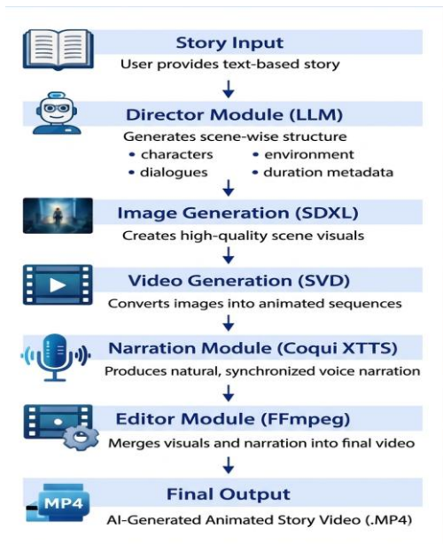
Fig. 1. System Architecture of STORYTALES
