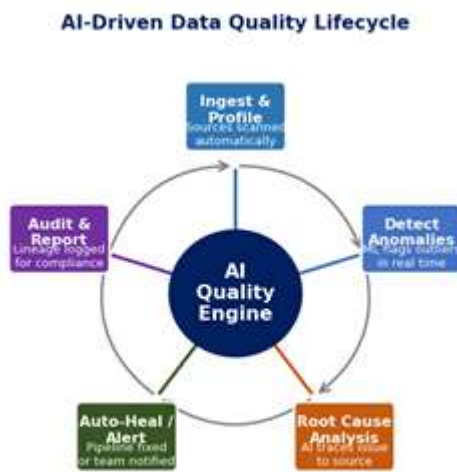
Fig. 2. AI-Driven Data Quality Lifecycle — five-stage continuous loop from ingestion profiling through anomaly detection, root-cause analysis, auto-healing, and compliance audit.
