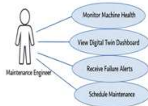
Figure 3: Use Case Diagram of Digital Twin Maintenance System
