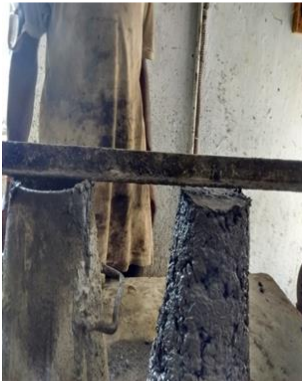
Figure 4. 1 Slump cone test
