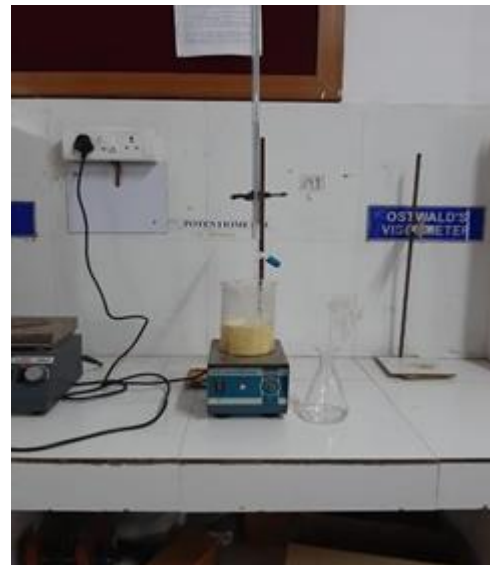
Figure 14: Titration of (NaOH) with (Ca(NO 3 ) 2 )
