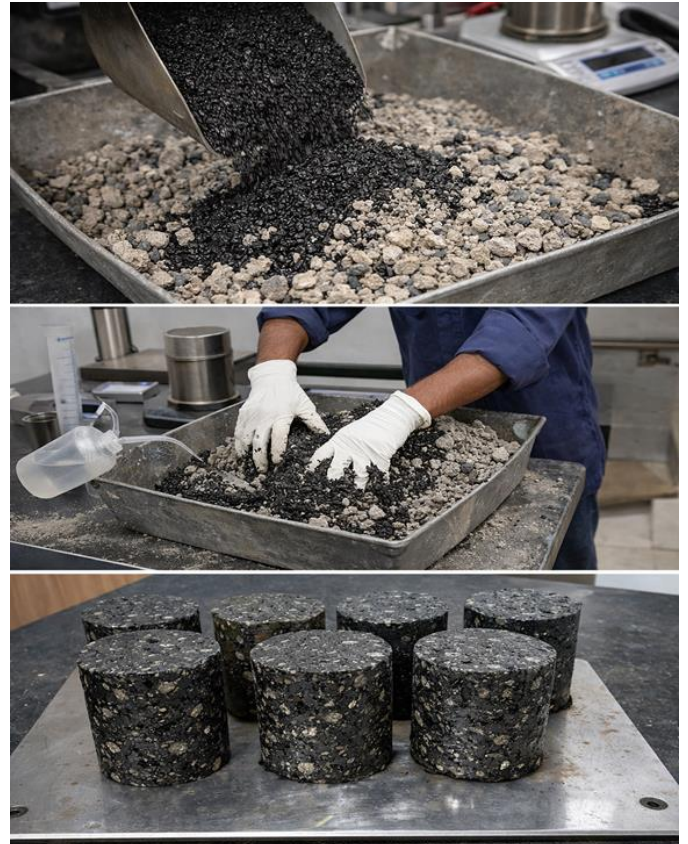
Figure 4.1: Preparation of rubber-modified specimens at Optimum Moisture Content
