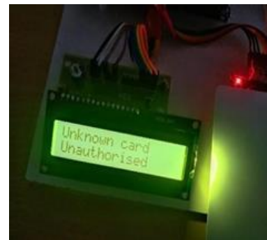
Fig 12. OTP entered is wrong and LCD displays as Unauthorised user.
