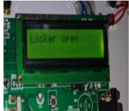
Fig 10.After entering correct OTP the box gets open
