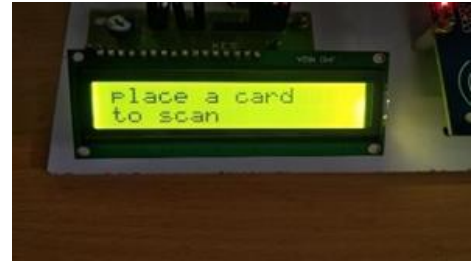
Fig 4. LCD display message to place RFID card
