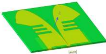
Fig. 8. 3D view of Vivaldi antenna with hexagonal and three rectangular slots
