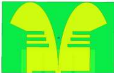
Fig. 9. Top view of Vivaldi antenna with hexagonal and three rectangular slots
