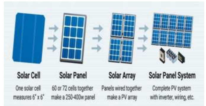
Fig 2 Solar PV system
