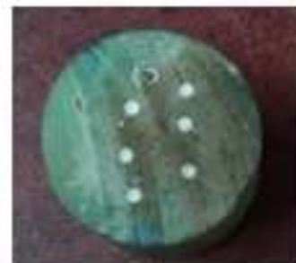
Figure 2: Hardness tested specimen
