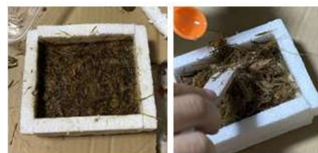
Fig. 7 & 8 Mixing of the samples with epoxy
