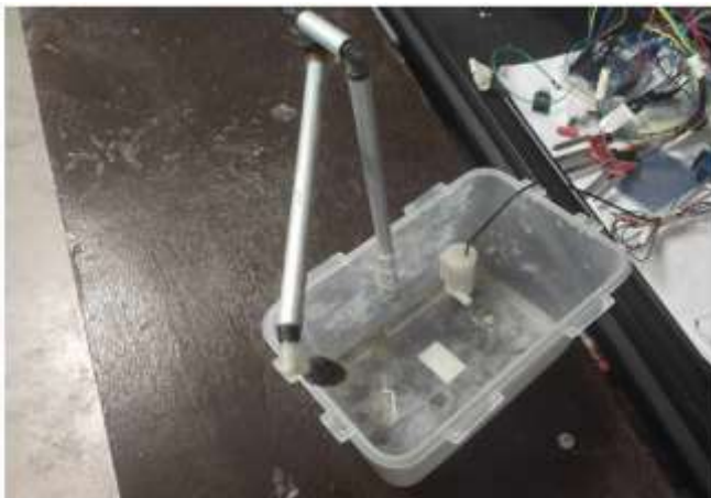
Figure 2. Submersible pump in the tank
