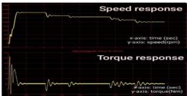
Figure 3: speed and torque responses of scalar control modelling with different input frequencies
