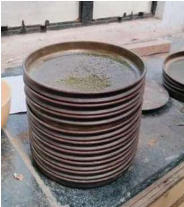
Fig. 3: Meshes of different grade from top to bottom with decreasing mesh holes for finer powder at each level
