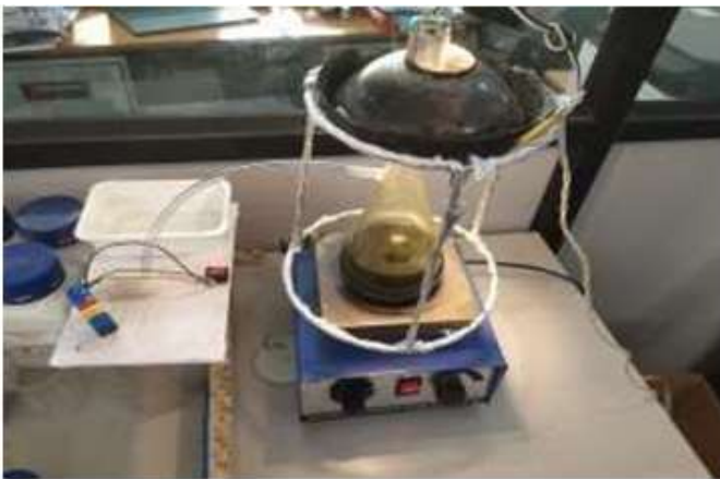
Fig. 4: Algae culture setup with photobioreactor, light source and carbon dioxide supply
