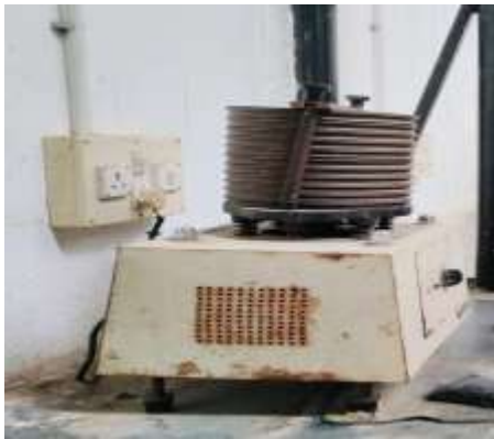
Fig. 2: sieve operated to produce fine powder of algae biomass for chemical pretreatment
