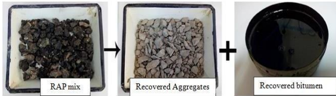
Figure 2: Recovered aggregates and Bitumen from RAP
