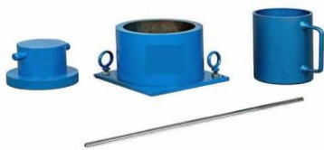
Fig 12 Crushing Strength Test.
