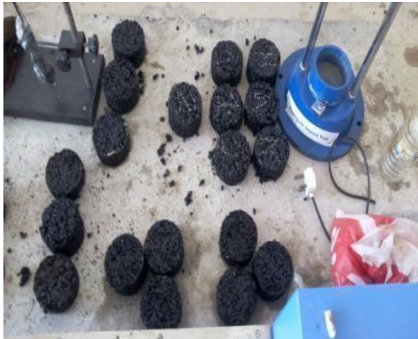
Fig 2. Blends of Aggregate and Bitumen and blends of Aggregate-bitumen- plastic mix.
