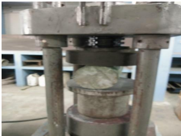
Fig 4. Tensile Strength Test Setup.
