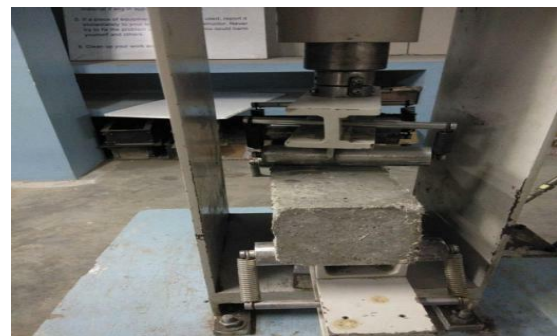
Fig 6. Test Setup for Flexural Loading.
