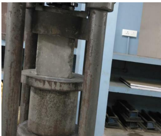
Fig 2. Uniaxial Compressive Strength Test Setup.
