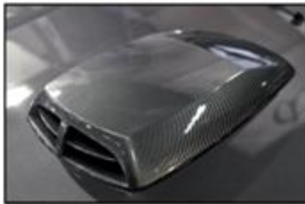
Fig 2 Example of polymer matrix composite used in the car hood.
