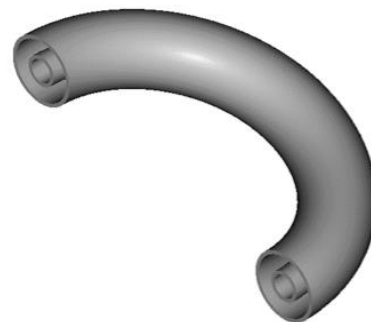
Fig.2: Close-up of double pipe coil
