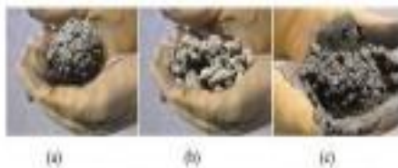
Figure 2.3 Workability of Pervious Concrete (Tennis et al. 2004)
