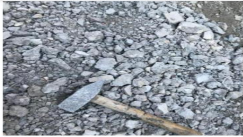
Fig. 2 Demolished concrete broken, and recycled aggregates obtained is processed for cleaning.
