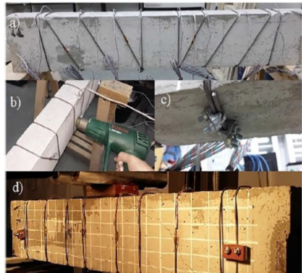
Fig 9. (a) Rear view of a strengthened beam, (b) activation process by means of heat gun, (c) detail of the anchoring using U-Bolt saddle clamps, and (d) front view of a beam with left and right outermost wire anchors [37].
