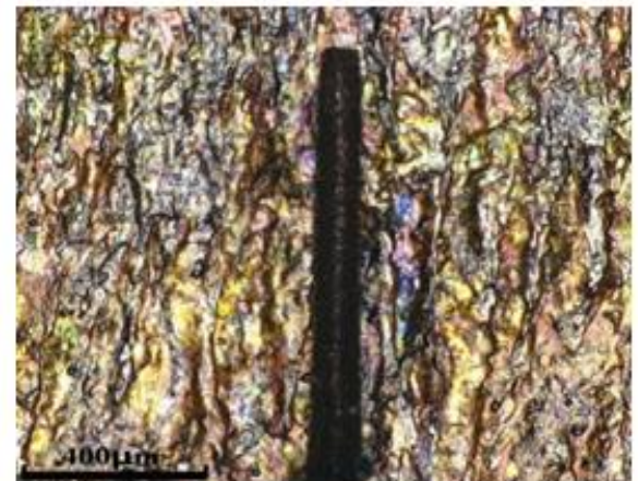
Fig 12. Micro-channel machined on copper sheet.
