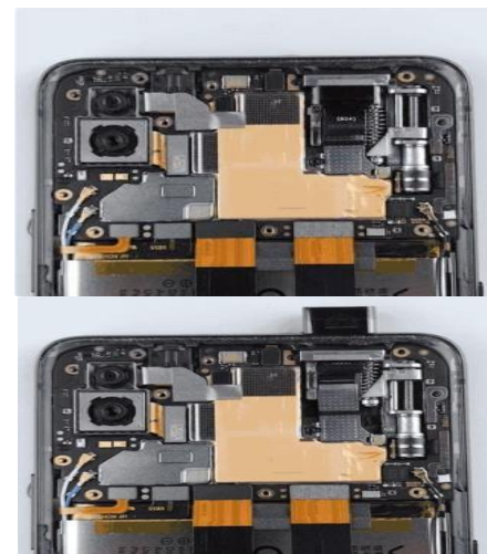
Fig 5. Step-4.1 Motorized Pop up Mechanism.
