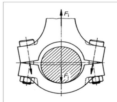
Figure 2 Horizontal close-in, bolt bending and gap opening caused by inertia force.
