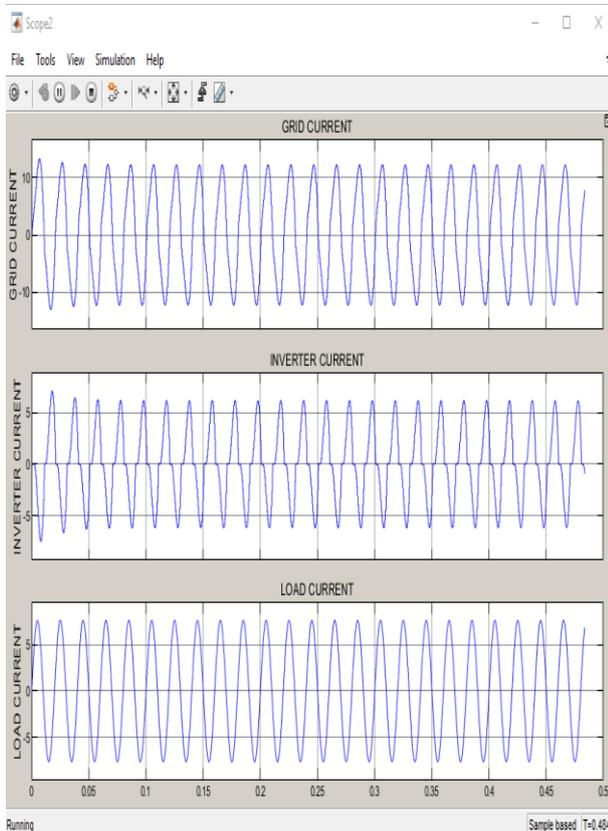
Fig 11. Grid, Inverter and Load Current.
